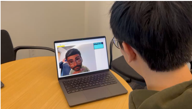
Figure 12. Real-time Web Rendering. Leveraging Gaussian Splats, our avatars efficiently render at 90–100 FPS on laptops and 30–40 FPS on mobile devices while occupying only 3 MB of disk space. In conjunction with a mobile face tracker, these avatars facilitate the creation of engaging filters and AR effects. The example shown features an avatar rendered in Google Chrome on an MacBook, developed in JavaScript.
